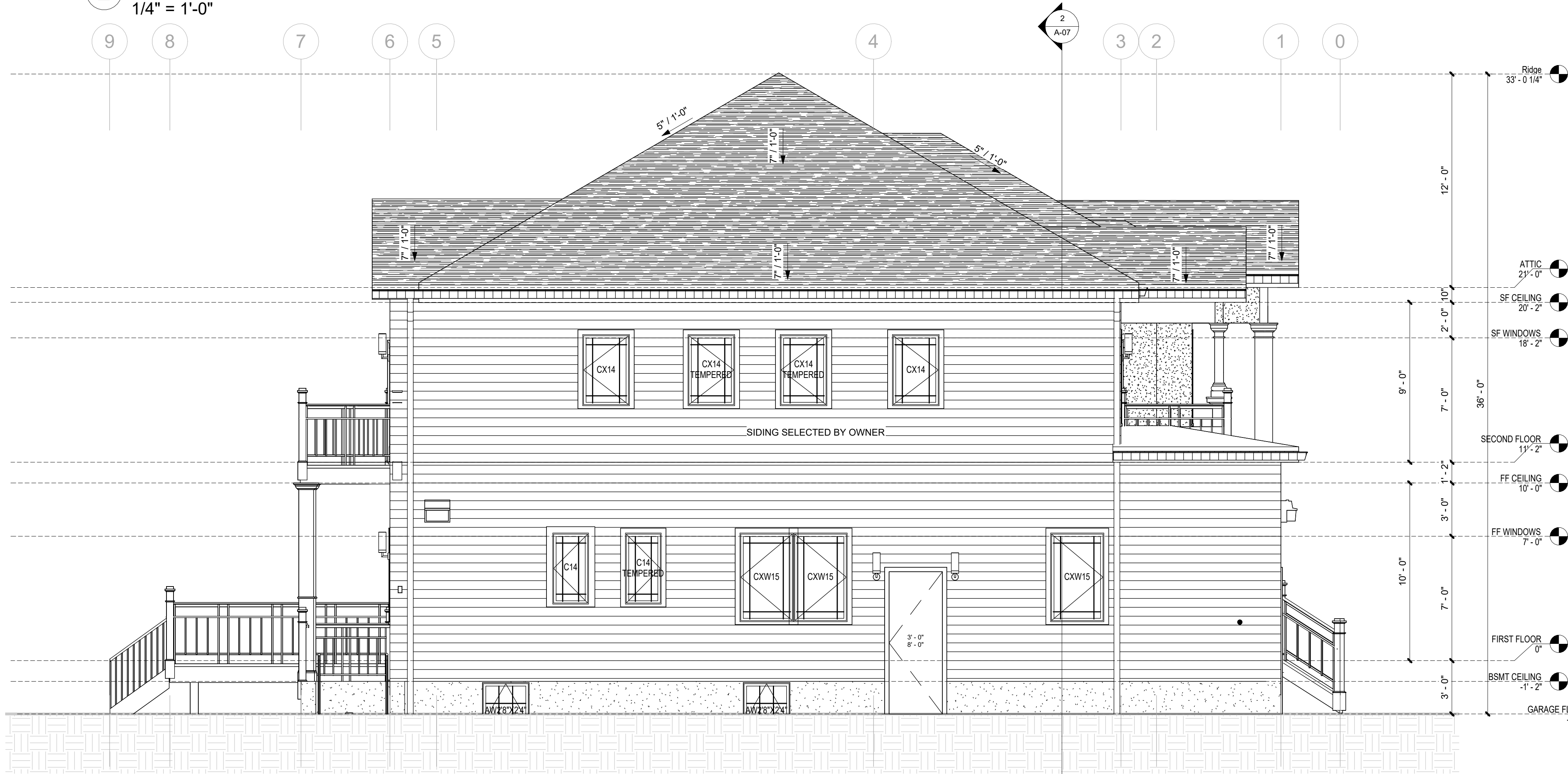
1 LEFT ELEVATION (SOUTH) 1/4" = 1'-0"
