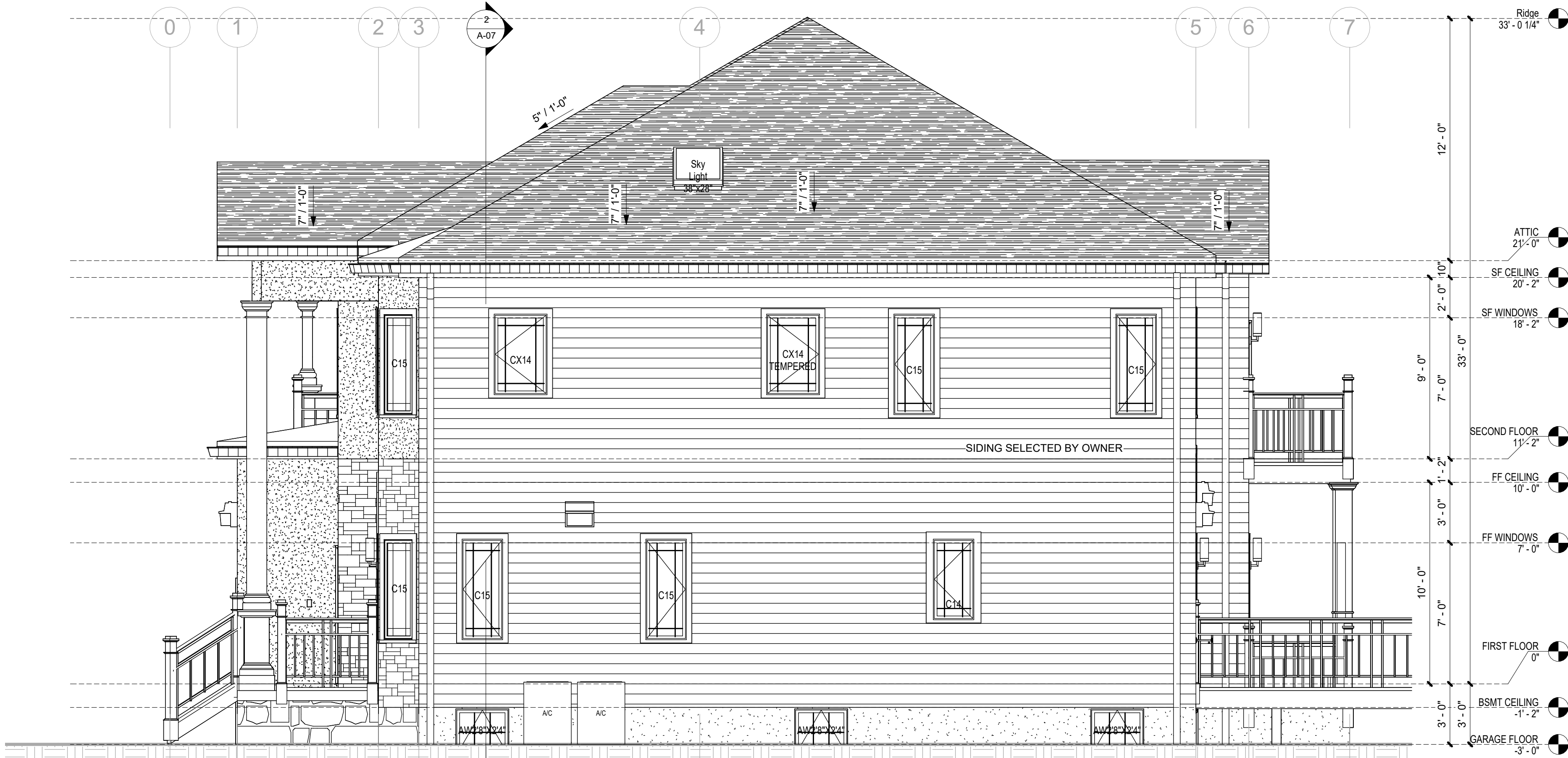
2 RIGHT ELEVATION (NORTH) 1/4" = 1'-0"
